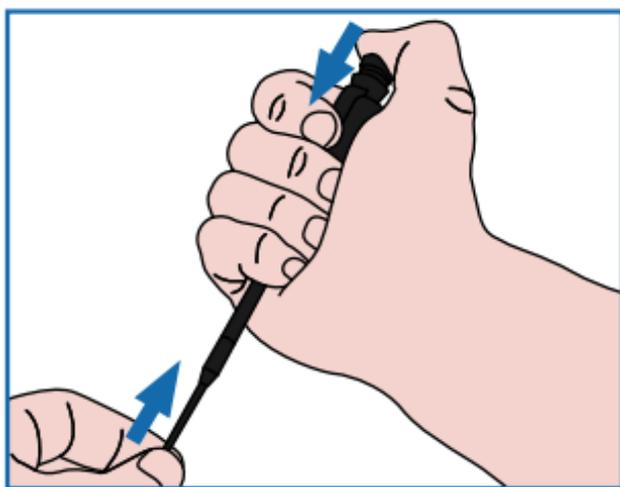
Press the button at the top of the pencil and insert the lead from the bottom.
