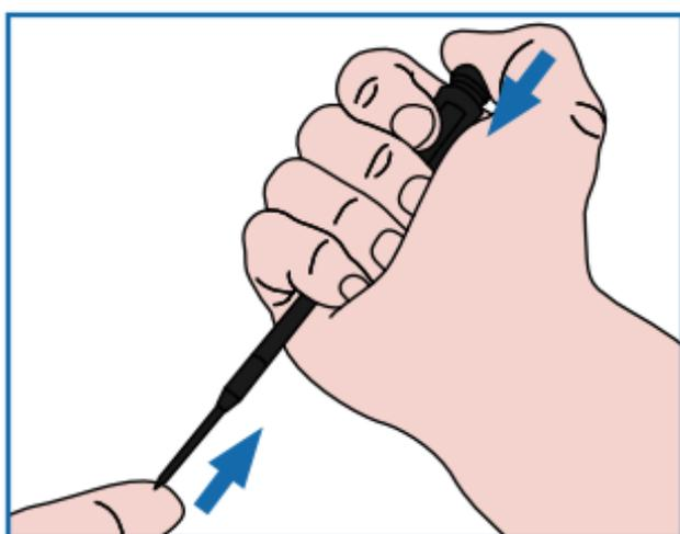
Keep the button pressed down and push the lead up to the desired level.
