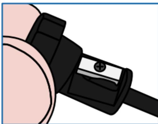
Sharpen the lead and screw the sharpener back onto the top of the pencil.
